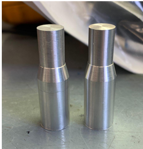
Figure 39: Machined clevis using a lathe
