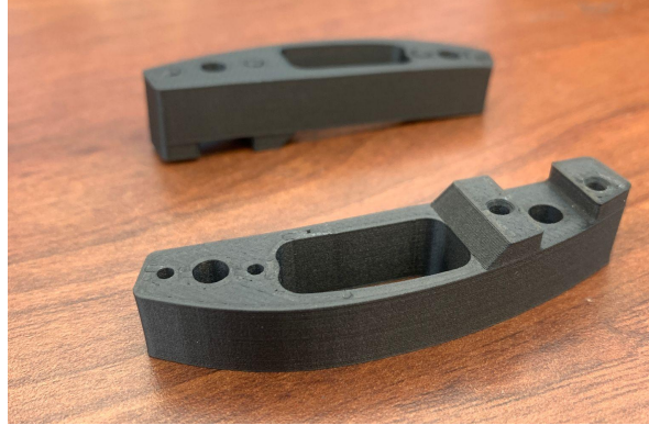
Figure 10: End caps 3D-printed in Carbon-Fiber Nylon
