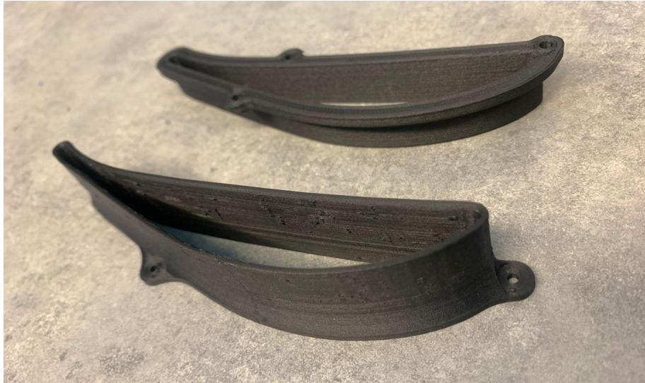
Figure 8: Foil sleeves 3D-printed using carbon fiber nylons
