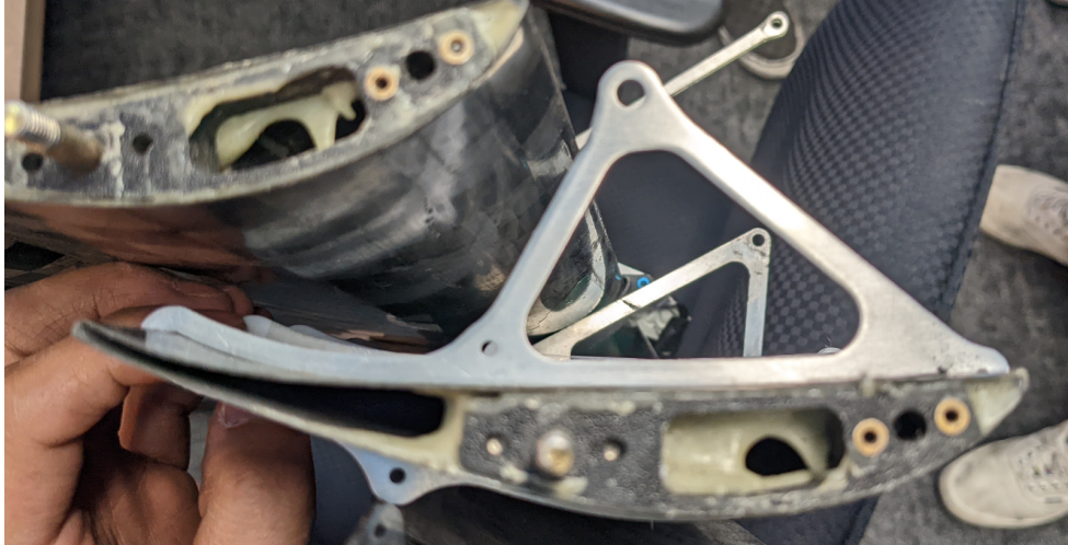
Figure 19: Sheet metal rear wing foil mount test fit on rear wing foil
