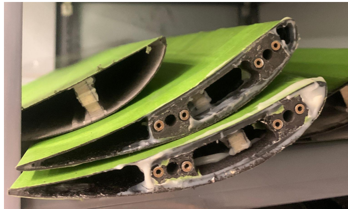
Figure 11: Bonded end caps on the side of the DRS airfoils
