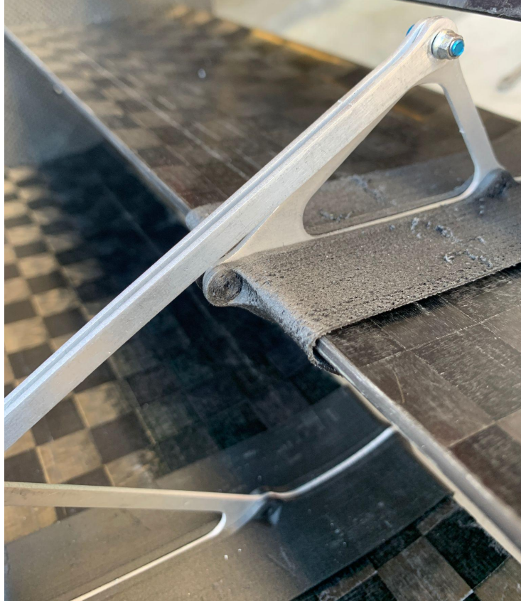
Figure 9: Foil sleeves assembled on the rear wing airfoils
